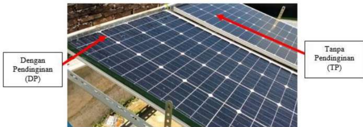
Gambar 1. Panel surya sistem pendingin
